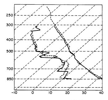
**Figure 6.** Radiosonde measurements of (right) temperature and (left) dew point temperature for a dry land area (dashed curve) and an irrigated area (solid curve) in northeast Colorado at 1213 local standard time (LST) on July 28, 1987. Reprinted from *Pielke and Zeng* [1989] with permission from National Weather Association.
