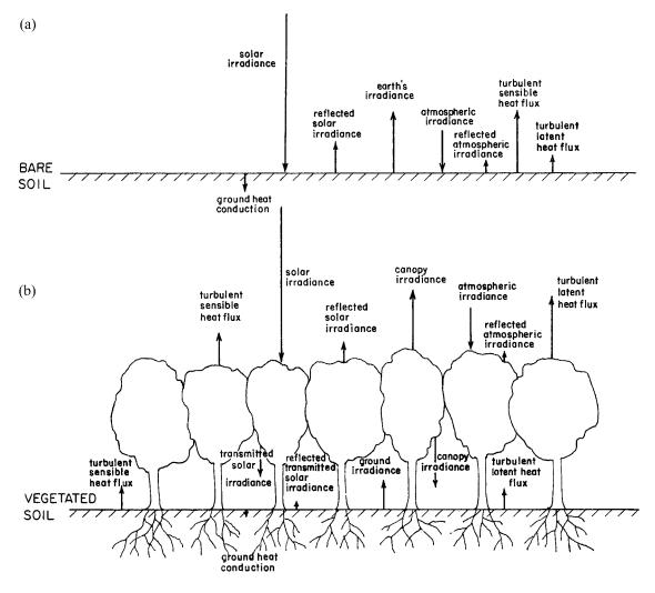
**Figure 1.** Schematic illustration of the surface heat budget over (a) bare soil and (b) vegetated land. The roughness of the surfaces (and for the vegetation, its displacement height) will influence the magnitude of the heat flux. Dew and frost formation and removal will also influence the heat budget. Adapted from *Pielke and Avissar* [1990] with kind permission from Kluwer Academic Publishers.
