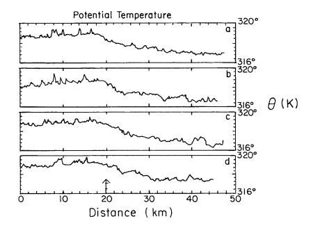
**Figure 7.** Measured potential temperature from Briggsdale to Windsor at the altitude of (a) 140 m, (b) 240 m, (c) 345 m, and (d) 440 m above the ground. The observed crop–dry land boundary is indicated by an arrow, with cropland to its right. Adapted from *Segal et al.* [1989] with permission from American Meteorological Society.
