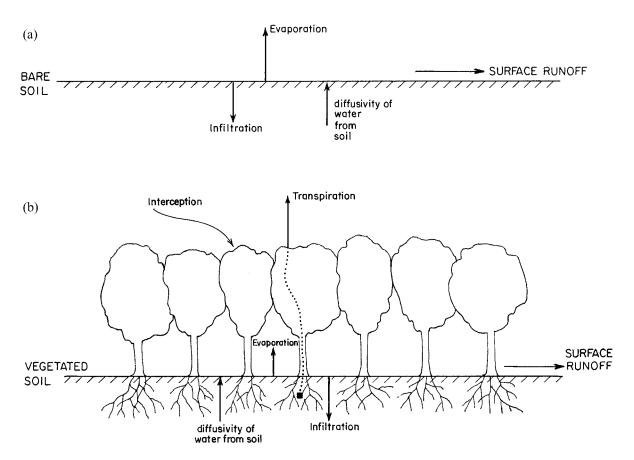
**Figure 2.** Schematic illustration of the surface moisture budget over (a) bare soil and (b) vegetated land. The roughness of the surface (and for the vegetation, its displacement height) will influence the magnitude of the moisture flux. Dew and frost formation and removal will also influence the moisture budget. Adapted from *Pielke and Avissar* [1990] with kind permission from Kluwer Academic Publishers.
