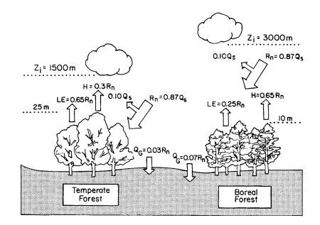
**Figure 4.** Schematic of the differences in surface heat energy budget and planetary boundary layer over a temperate forest and a boreal forest. The symbols used refer to equation (1). Horizontal fluxes of heat and heat storage by vegetation are left out of the figure. Adapted from P. Kabat (personal communication, 1999). Reprinted with permission.
